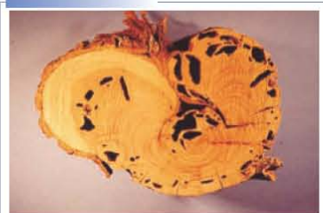
Dry wood Termite attack
