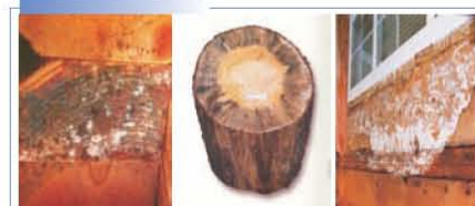
Mold and fungi attack on wood.
