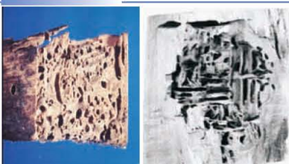
Carpenter ant attack; nesting galleries usually cut across grain and are free of residue.
