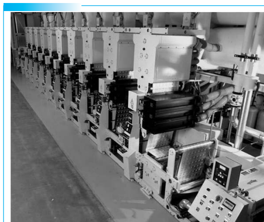
Fig 2: Interstation UV installation on a Flexo Press
