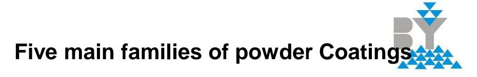
• **Epoxy-polyester hybrid** powder coatings are epoxy powders with a high percentage of polyester resins (some-times approaching or exceeding 50%). These powders are similar to epoxies with improved resistance to yellowing in sunlight and weatherability. Hybrid powders are considered the backbone of the powder coatings industry and make up 51% of world powder production.
